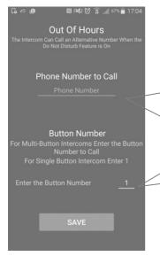
For commercial installations, sometimes it is desirable to call an alternate number after the "do not disturb" watershed time. If a phone number is entered in this screen, then the intercom will call the previously programmed standard numbers during normal operating times, and this alternate phone number after hours
