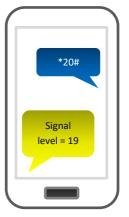
Note: Reception levels below 14 can cause problems with DTMF relay control, poor quality audio, no audio coming from the microphone on the intercom (the person on the phone cannot hear anything), or buzz on the loud speaker.
