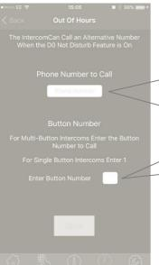
For commercial installations, sometimes it is desirable to call an alternate number after the "do not disturb" watershed time. If a phone number is entered in this screen, then the intercom will call the previously programmed standard numbers during normal operating times, and this alternate phone number after hours
