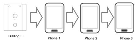
Any user receiving the call can answer, speak to the visitor, and press the following digits on their mobile or fixed line telephone to control the relays on the device...
