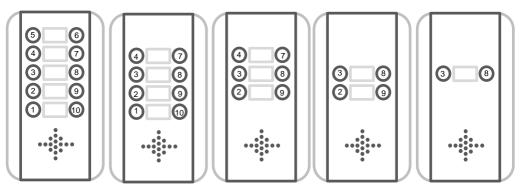
Please note the position of the buttons on the above panel options. For example, if you have a 2 button panel, you will be programming dial out numbers for buttons 3 and 8. For a 4 button panel, the corresponding button locations are 2,3,8 and 9.
